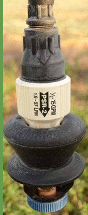
LEPA Low-elevation shroud
