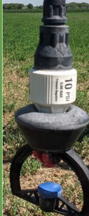
LESA Low-elevation spray
