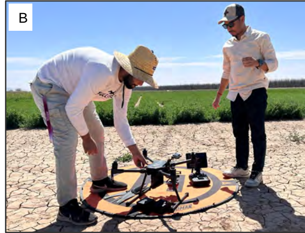
Figure : A. NMSU Alfalfa Breeding drought study with water smart alfalfa germplasm, B. UAV preparation for capturing reflectance from the water smart alfalfa germplasm; UAV is DJI Matrice 210 mounted with Micasense altum sensor
