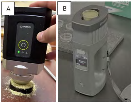
FIGURE 1 Samples being scanned with two portable handheld spectrometers. Trinamix spectrometer (A) in direct contact with the sample (ground to pass a 0.04-inch screen); NeoSpectra spectrometer (B) with the sample (ground with a cyclone mill) in a sampling container provided by the manufacturer.
